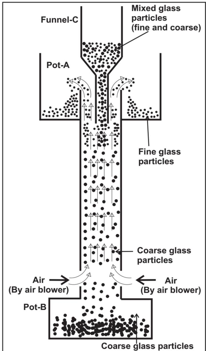
Air was thrust by the air-blower from below the vertical pipe through a number of big holes. Mixed glass particles were put in the funnel. Because of the thrust of the air, fine particles were pushed upward and collected in the pot (A) and the coarse (big particles) fell at the bottom and were collected in the pot (B).
